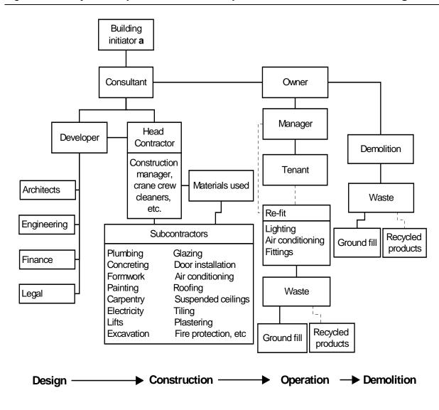
Figure B.1 Stylised representation of the phases of a commercial building
