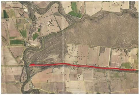
Above: Areal view, TIA Channel 2/4/1 > 3km (red line) showing vegetation on both sides of the channel. This channel was constructed to pump water using steam driven pumps from the Murray River into Gunbower Creek. The cannel was dug out by men using teams of horse-drawn scoops in 1900c.
