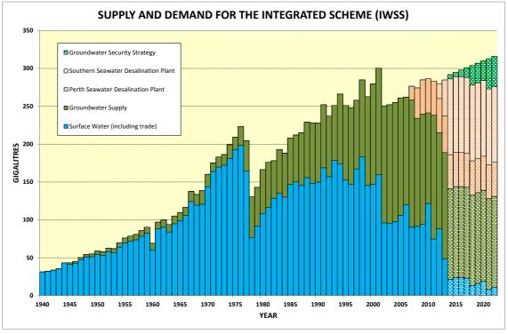
Figure 8: Water sources for the Integrated Water Supply System (1940-2023)<sup>151</sup>
