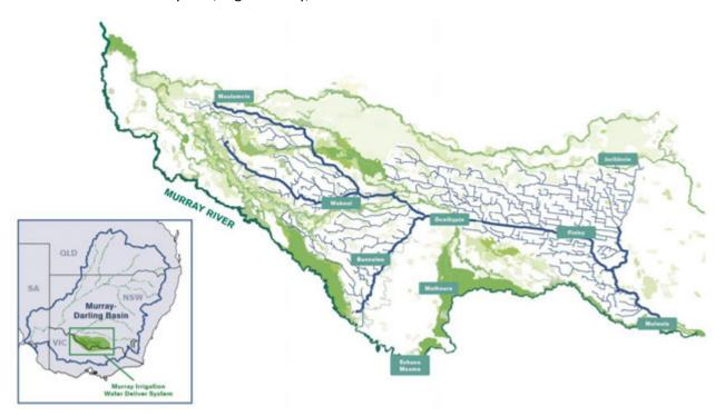
Figure 1. Murray Irrigation Limited water delivery network in the Southern Murray Darling Basin.
