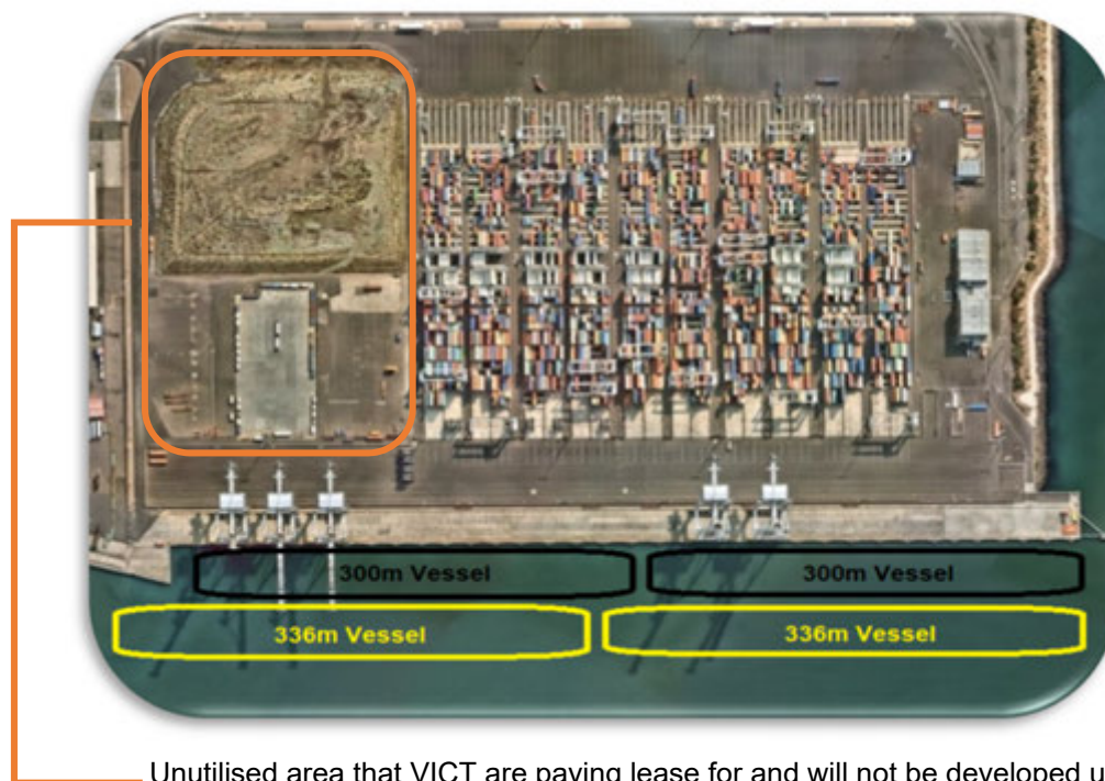
Image 1.2 – VICT's berth length design with two 300 meter vessels compared to the current 336 meter vessels calling at the Port of Melbourne:
