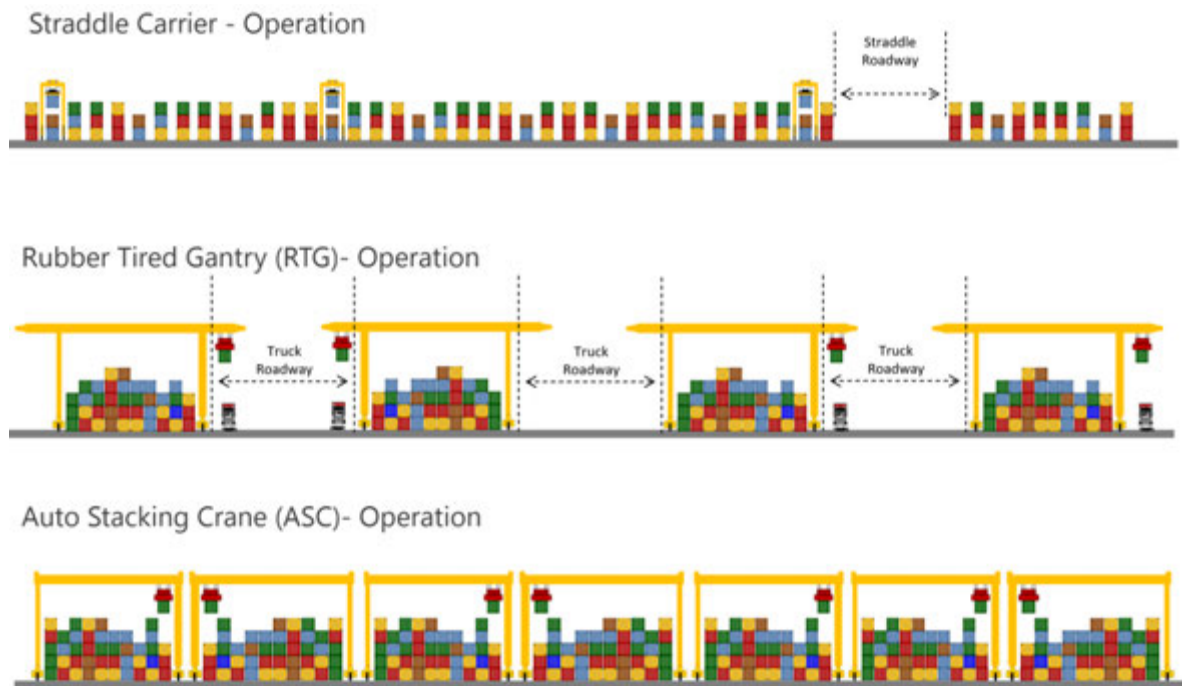
Figure 9: Various Terminal modes of operation. Presently Adelaide operates a Straddle Carrier (S/C) operation which offers the least capacity of all the modes. Sometime in the near future the terminal will look to change this mode to allow for a far greater capacity.
