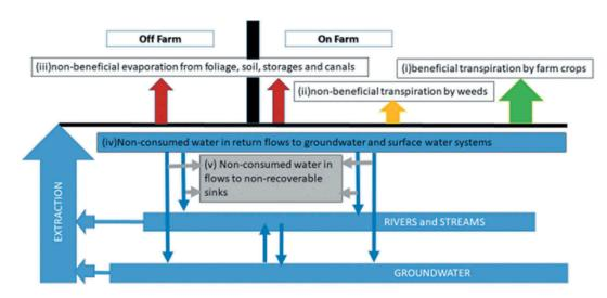
Figure 1. Water flows associated with irrigation.
