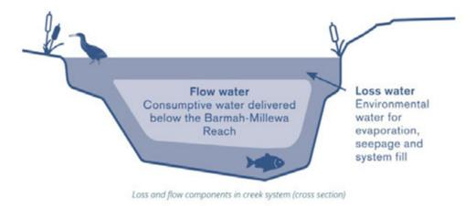
Figure 3: Diagram outlining how MDBA river operations water can be used as the "flow" water while Held Environmental Water covers the "loss" component, working together to achieve an environmental outcome in an ephemeral creek system.
