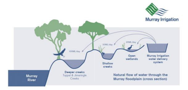
Figure 2. Cross section showing how MIL's water delivery system is positioned in the landscape relative to nearby rivers, creeks and wetlands.
