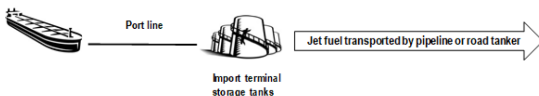
FIGURE 2.3 GENERAL ARRANGEMENT FOR AN IMPORT TERMINAL
