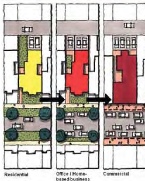
An example of how a well-located and configured lot can enable its use to evolve from residential to home-based business use, and then to full commercial use
