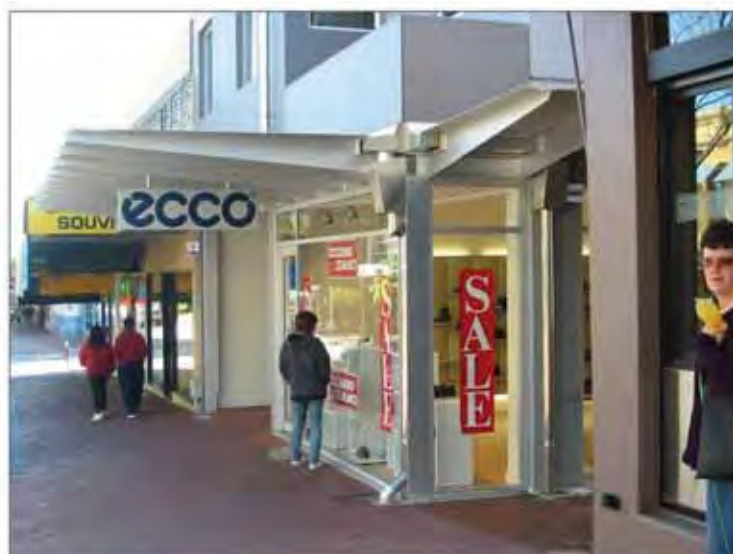
An example of good “active” building frontage with full-height display windows at street level and doors opening directly onto the street.
