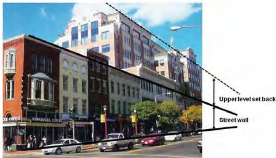
An example of how the upper levels of larger buildings can be setback to enable the lower levels to establish a street wall of a scale that complements the character of the place.
