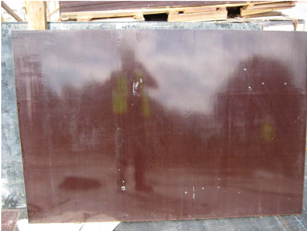
Plate Four – Upper face of formwork plywood sheet – no brand
