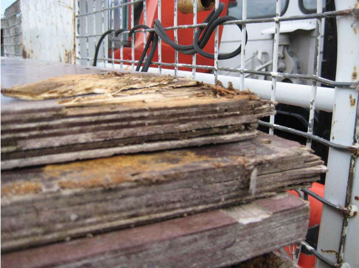
Plate Three - Pack of formwork plywood showing delamination on edges
