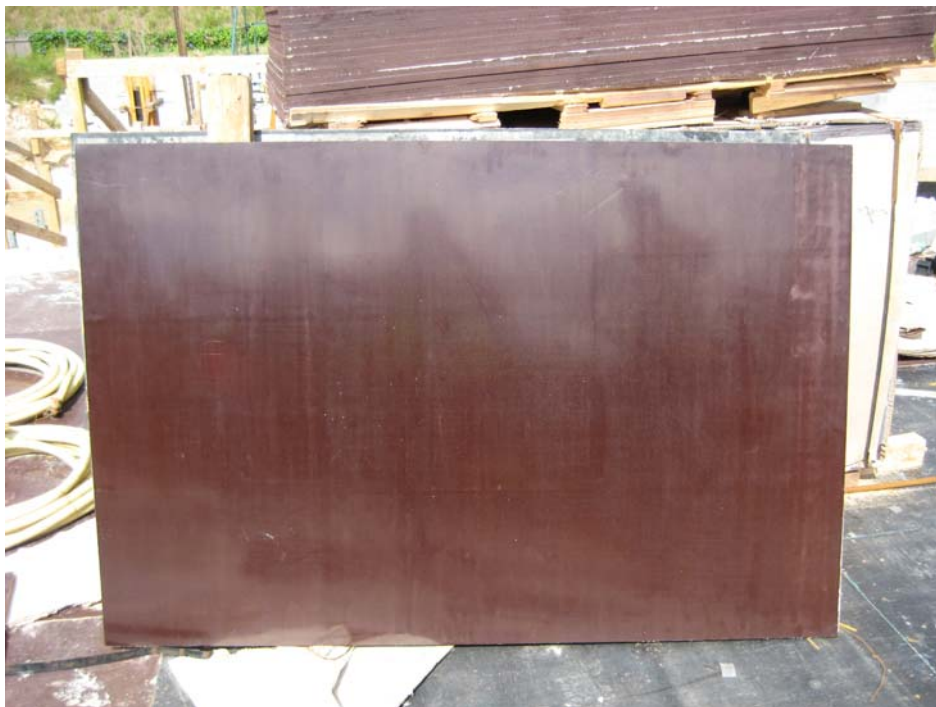
Plate Five – Bottom face of formwork plywood sheet – no brand
