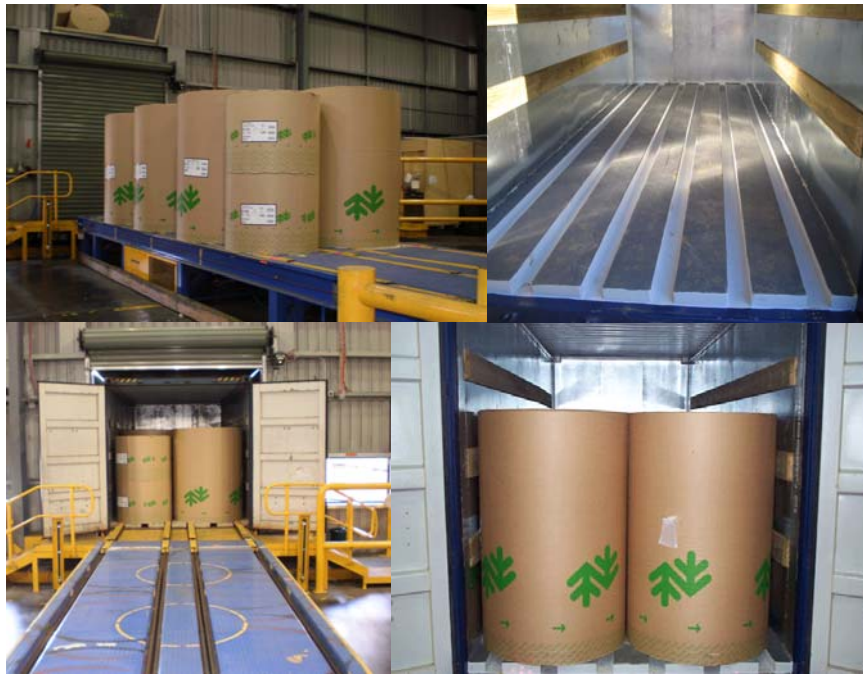
Fig 1. S-Box Loading Bay at the Boyer Mill highlighting skate loading facility.
