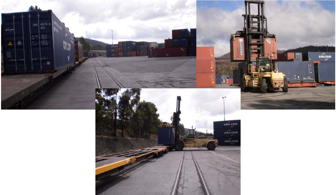
Fig 2. Shipping units assembled on warehouse “hardstand” ready for loading of daily train to Burnie Port. 40 foot forklift loading TasRail train prior to departure and transit to Burnie
