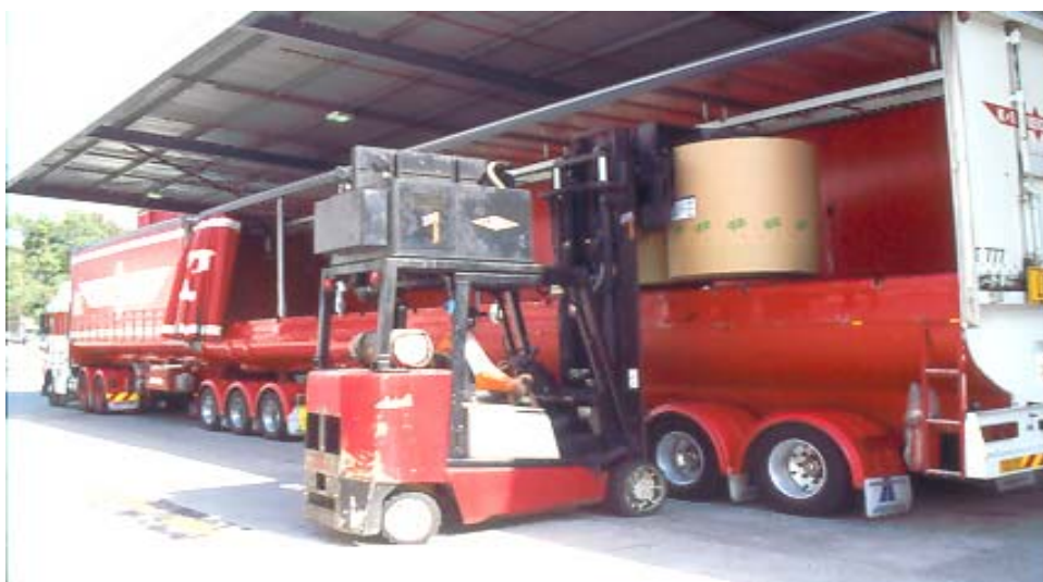
Fig 8. Truck/trailer (MEPA) transports chemicals (lower layer) to the Albury Mill and then back loads with Paper.
