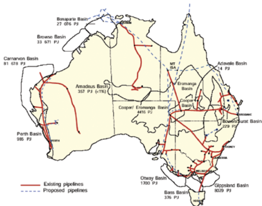
Figure 21 Australian Natural Gas Reserves and Gas Transmission Pipeline Infrastructure
